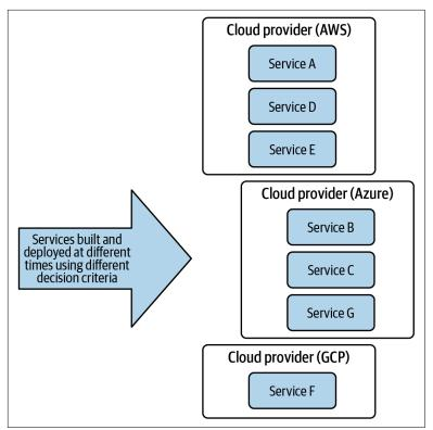
*Figure 2-6. Independent deployment decisions made at different times (Service A through Service G)*
