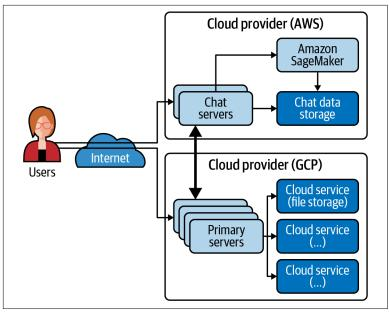
*Figure 3-5. AI/ML capabilities offered by specific cloud providers can lead to polycloud*
