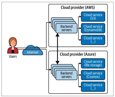
Figure 1-3. Simple multicloud deployment
